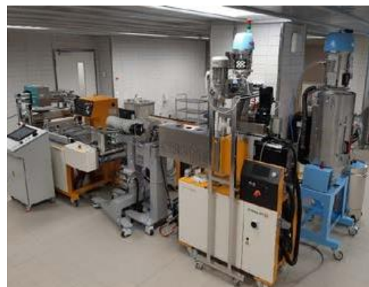
Pilot scale compounder & flat film extrusion line
