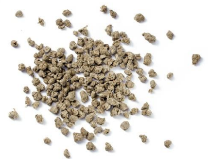
AgriPlast – A composite made of plastics and cellulose fibres
