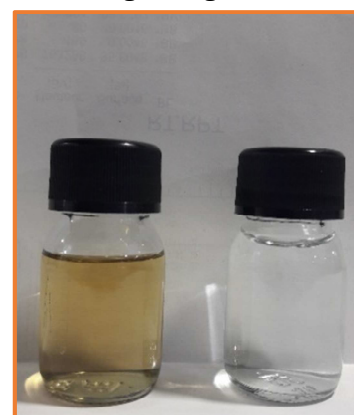
Bottom Purification pilot plant: left: Crude MMA, right: Regenerated MMA.
