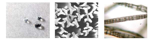
Plant-based fibre solutions for AHP products: the hydrophobized Olea fibre for the topsheet, the trilobal Galaxy<sup>®</sup> fibre for the acquisition/distribution layer and the hollow Bramante fibre for the absorbent core.
