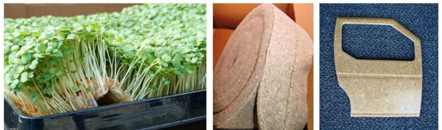
Left to right: Hemp fibre bounded with PLA-fiber a growth medium for spicy herbs, nonwoven hemp fibre mats, reinforced bio-composite. Pictures: Bodil Pallesen.
