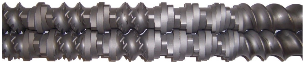
Figure 4: different screw elements of a twin screw extruder
