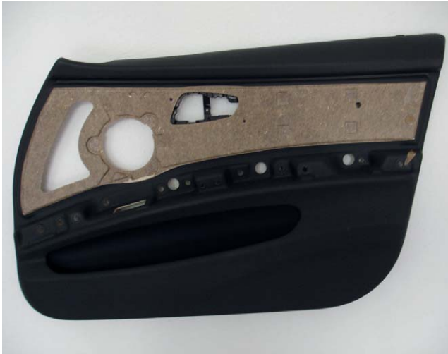
Door panel made of natural fiber/PP
