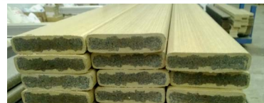
Multilayer WPC-decking boards with recycled ABS (45%) + wood (55%) inside and recycled PE or PP (35%) + wood (65%) outside
