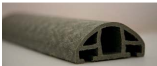
Decking manufactured with dry blend (micronized hemp chaff)
