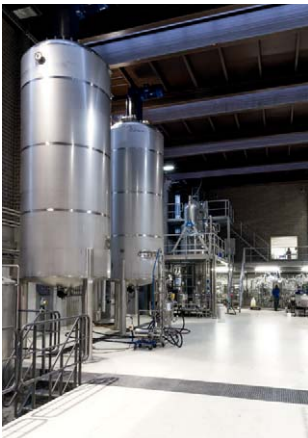
Equipment for scale-up of fermentation processes. Bioreactors with a volume of 7 l to 15,000 l.
