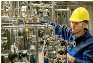
Equipment for scale-up of fermentation processes. Bioreactors with a volume of 7 l to 15,000 l.
