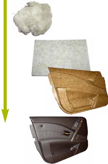
Natural fibre door panel for BMW 5 Series, compress moulding (Germany). Pictures: nova-Institut
