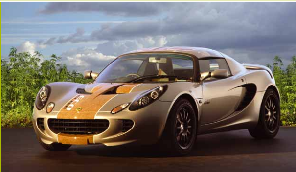
Sports car Lotus Eco Elise, in the main made from different natural fibre compounds, hand lay-up, vacuum bagging and RTM (UK). Picture: Lotus Cars
