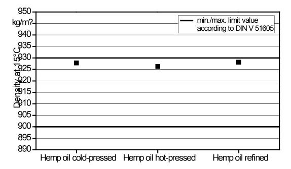
Figure 5: Density at 15 °C (EN ISO 12185) of different samples of hemp oil
