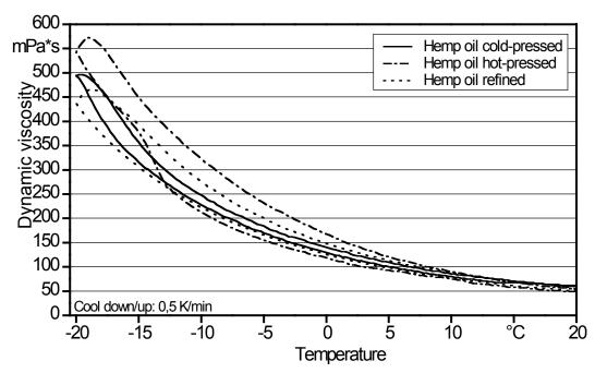
Figure 4: Dynamic viscosity of different samples of hemp oil, measured by a rotation viscosimeter, with a cool down/up speed of 0.5 K/min
