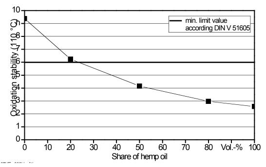
Figure 26: Influence of the share of hemp oil on the oxidation stability (110 °C) (EN 14112) of a mixture of hemp oil and rape-seed oil
