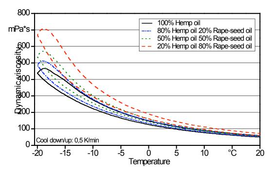
Figure 24: Dynamic viscosity of mixtures of hemp oil and rape-seed oil, measured by a rotation viscosimeter, with a cool down/up speed of 0.5 K/min
