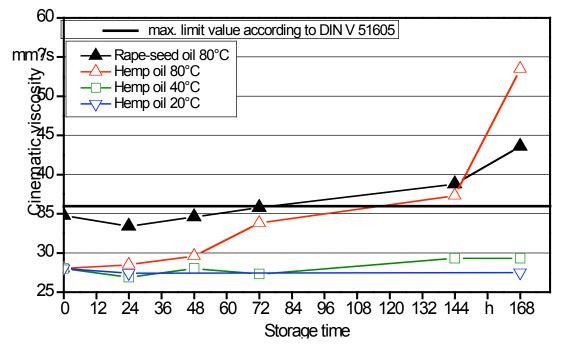
Figure 21: Change of kinematic viscosity (40 °C) (ISO 3104) of hemp oil and rape-seed oil stored at different temperatures
