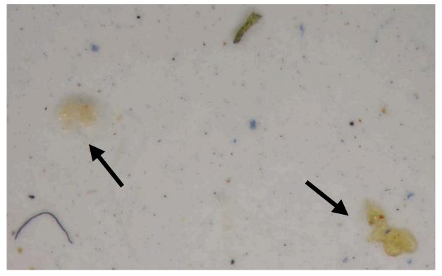
Figure 2: Particles from polymerised hemp oil on the filter membrane of the sample "hemp oil cold-pressed" before conditioning, shown by a microscope
