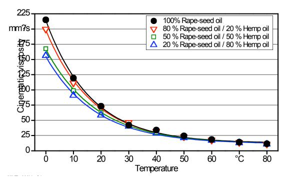
Figure 22: Temperature depended behaviour of cinematic viscosity (ISO 3104) of mixtures of hemp oil and rape-seed oil
