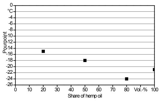
Figure 25: Influence of the share of hemp oil on the pour point (ISO 3016) of a mixture of hemp oil and rape-seed oil
