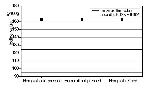
Figure 11: Iodine value (EN 14111) of different samples of hemp oil
