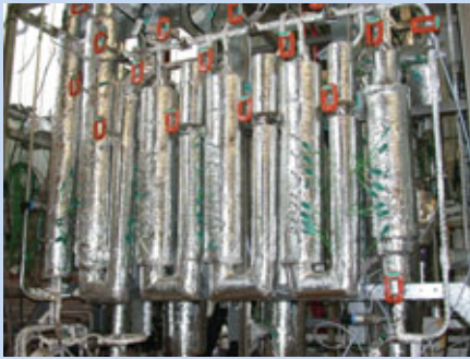
Fixed bed SNG reactors at ECN with thermocouples to measure temperatures at eight positions in each reactor.
