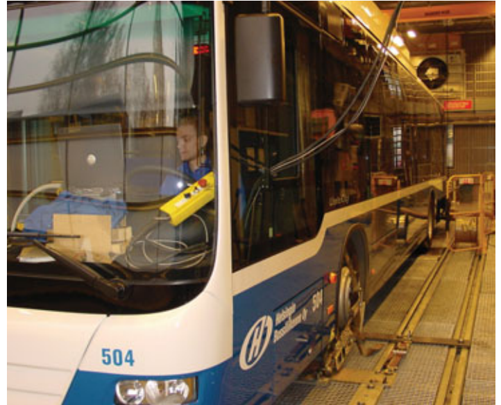
The heavy-duty chassis dynamometer is used to measure fuel consumption and emissions in large vehicles
