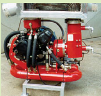
Joanneum's biomass driven Alpha-type Stirling Engine, 3kWel
