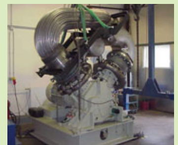
Joanneum's biomass driven Alpha-type Stirling Engine, 30kWel
