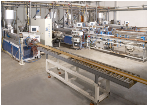
Six extrusion lines for the production of wood polymere composites. The twin-screw extruders „Bitruder“ from Reifenhäuser serve as a basis for these plants. (Source: Reifenhäuser)
