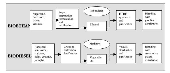
Figure 1: Biofuel manufacturing processes
