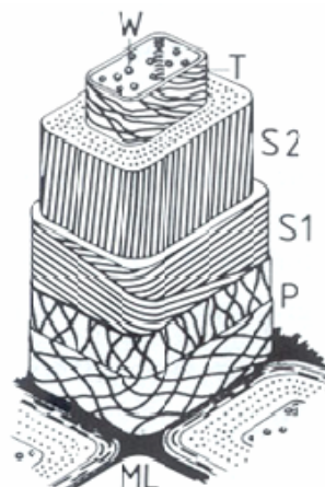
Figure 2 Model of a softwood tracheid cell wall showing the different cell wall layers.
