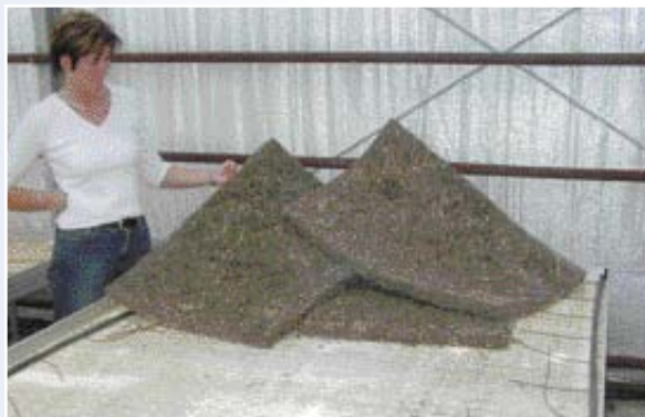
Seegrasmatten aus Sakskøbing, DK Insulation mats made of sea grass in Sakskøbing, DK
