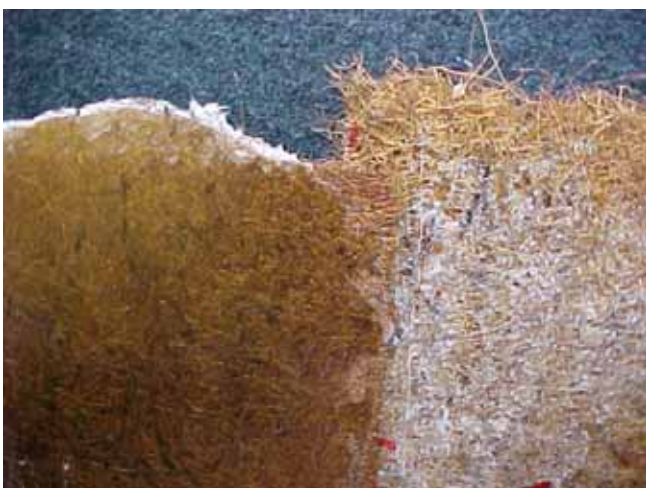
PMMA-Coir, consolidated sheet (left) and the prepreg (right)
