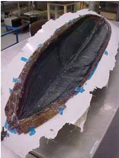
final product in the mould (left) en just released from the mould (right)
