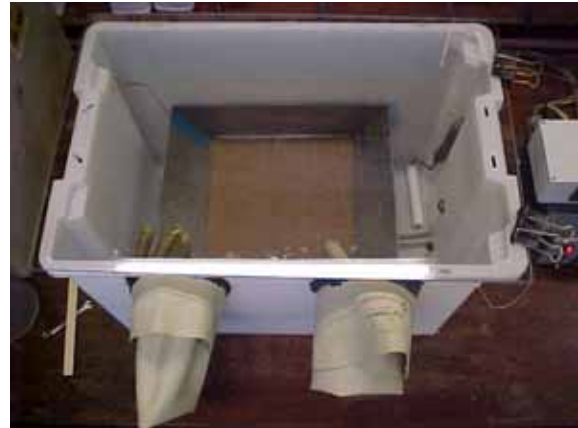
The nitrogen filled box
