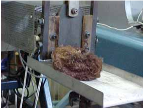
The coir fibre-PP mixture comes out of the extruder
