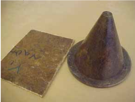
On the right the LFT-compressed cone
