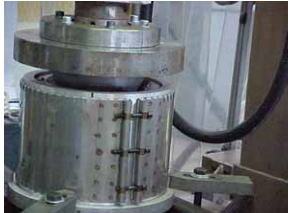
The lump is put in between two moulds and compressed
