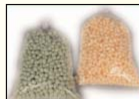
AGRIPACK packaging material from maize starch
